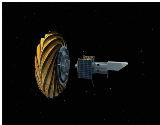
**Fig [4]:** The initial phase of sail separating from housing and then in the process of expansion, courtesy-SEEKER.
